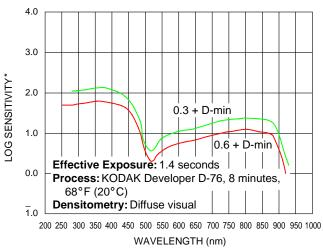
\*Sensitivity = reciprocal of exposure (ergs/cm²) required to produce specified density
